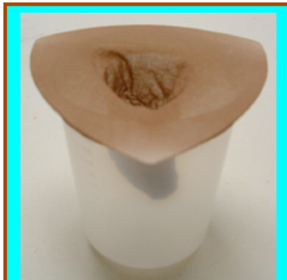
The fast-flow nylon filter makes it easy to separate the cellular matter from the buffer.
